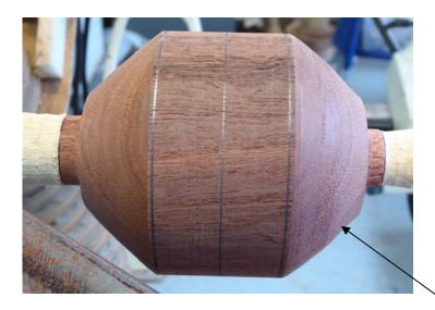
Take care not to remove to much material at the centre point as this is the finished size of the sphere
