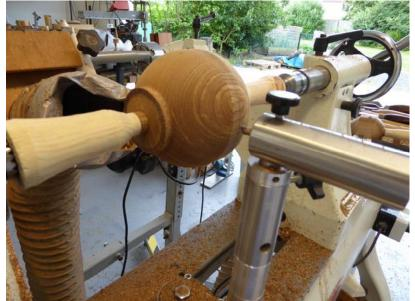
Start turning the by advancing the cutter taking light cuts .
