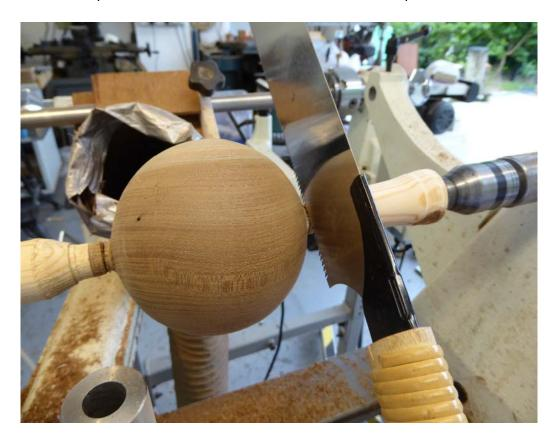
Mount the sphere between a pair of cup chucks with the stubs offset to each other, turn each stub off taking care not to cut into the sphere. (I find a sharp bowl gouge very good for this operation) Us as large as possible cup chuck at the spindle end as this will help to make the sphere run true
