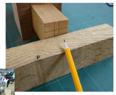
Mount between centres and turn to a cylinder 100mm diameter
