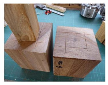
This is to make a 100 mm (4") Sphere. Cut your 100mm timber to about 110 long and mark the ends as shown above ready to hot melt glue scrap blocks to each end. Using scrap blocks save wasting good timber.
