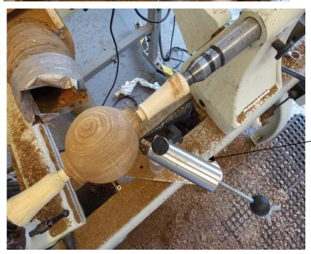
To get closer to the end points rotate the cutter head a few degrees as shown and then advance the cutter again taking light cuts. Finish one end and then repeat for the other end offsetting the cutter head in the other direction.
